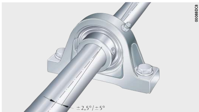
Figure 1 Compensation of static shaft misalignment
